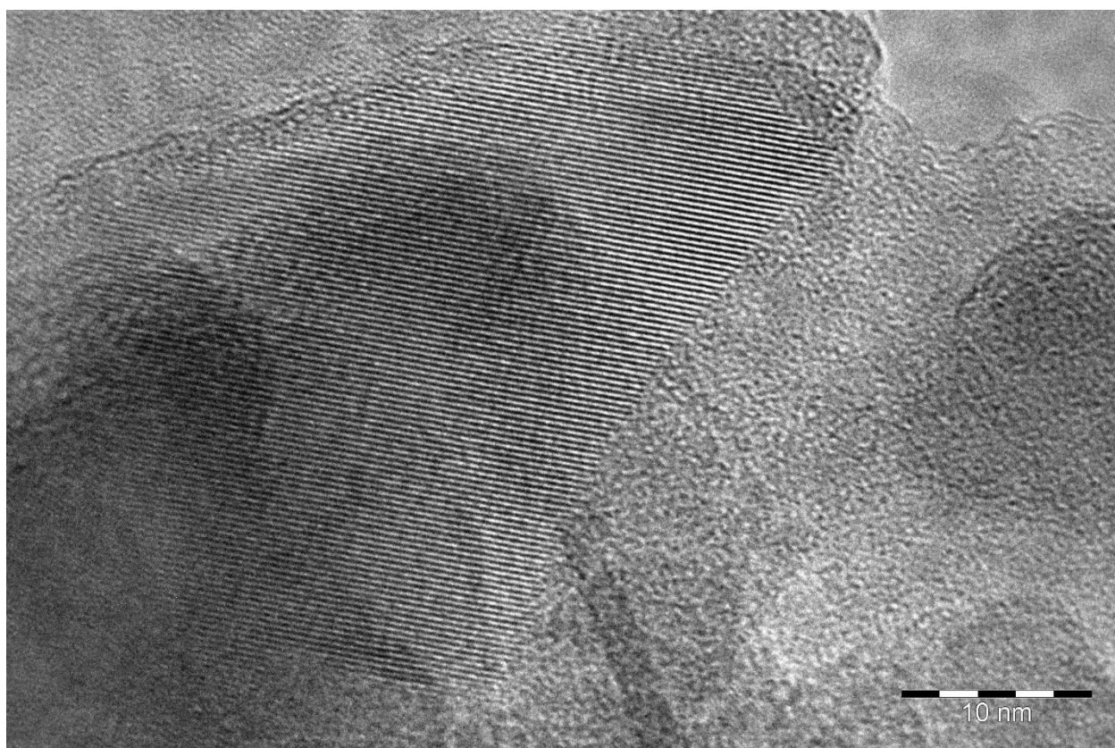
Figure S3 HR TEM image of a crystallite in the sample, cycled through Si/SiP transition 10 times.
