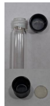
Figure S1 Reaction vessel for the optimization studies
