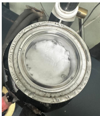
Figure 1 Carbon dioxide hydrate obtained from CO 2 and a 1% lithium chloride solution.
