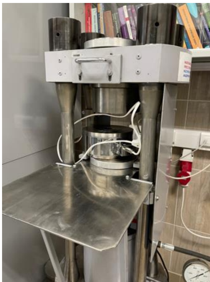
Figure S3. Cell with a piston-cylinder chamber.
