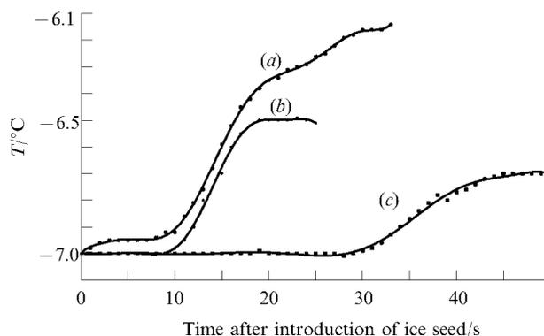
Figure 2 Effect of the surfactant  $\gamma$ -aminopropyltriethoxysilane on the temperature-time dependencies during ice nucleation with (a), 0 (reference solution); (b), 1; (c),  $10 \text{ g dm}^{-3}$  of surfactant.
