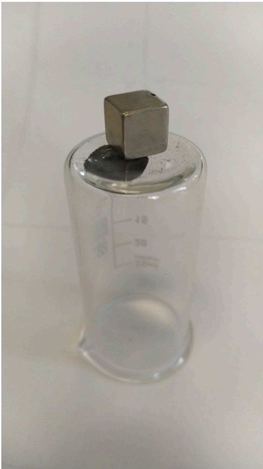
Figure S2. Ferromagnetic properties of activated Ni catalyst.
