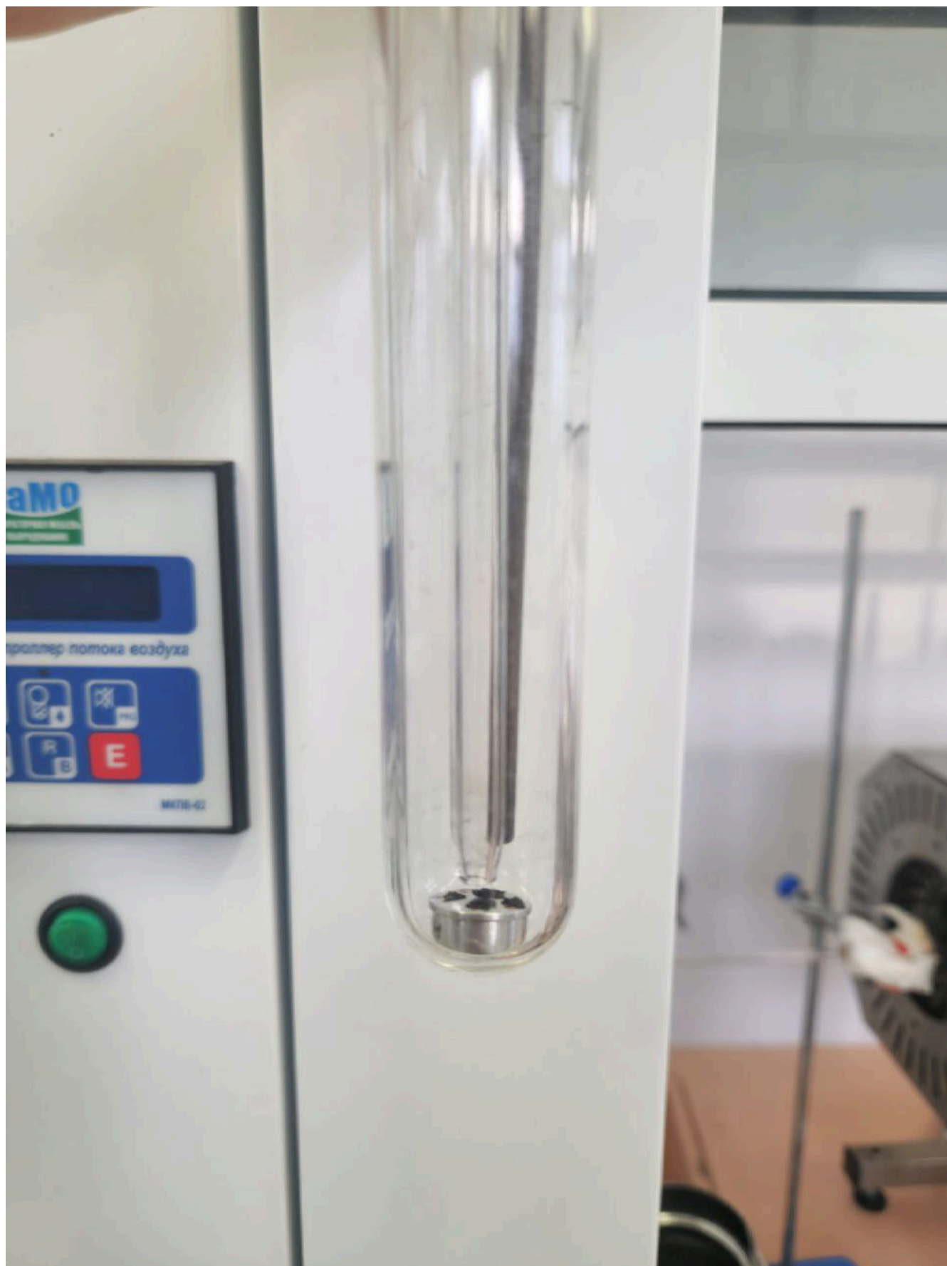
Figure S1. Samples on microscopy stub in the reactor.
