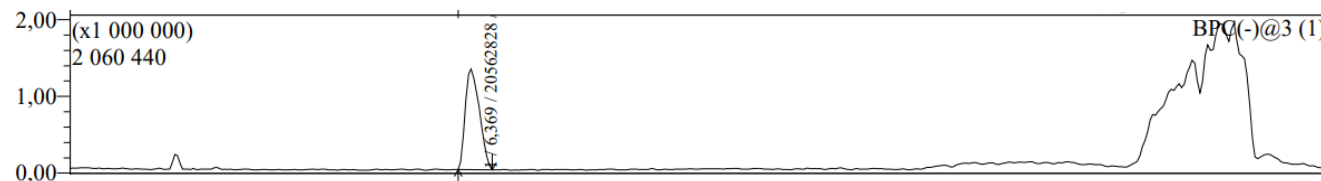
LCMS chromatogram of 2e : MS detection of - ions
