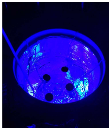
Figure S5. Photoreactors used in the study (left) and the interior view of the reactor (right). The reactors equipped with blue LEDs are shown.
