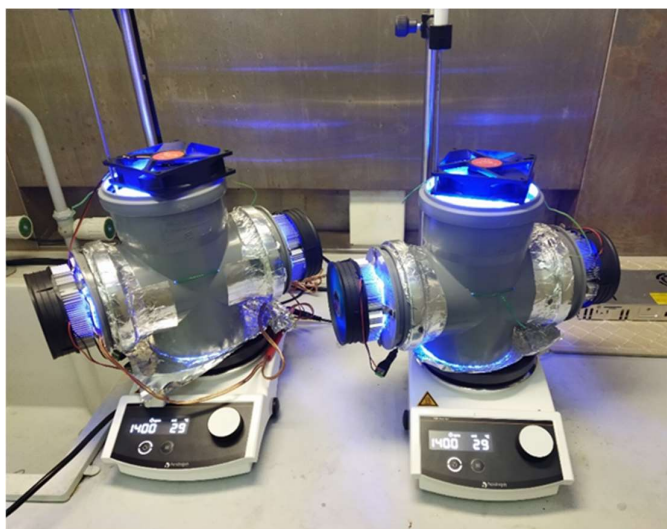
Figure S5. Photoreactors used in the study (left) and the interior view of the reactor (right). The reactors equipped with blue LEDs are shown.
