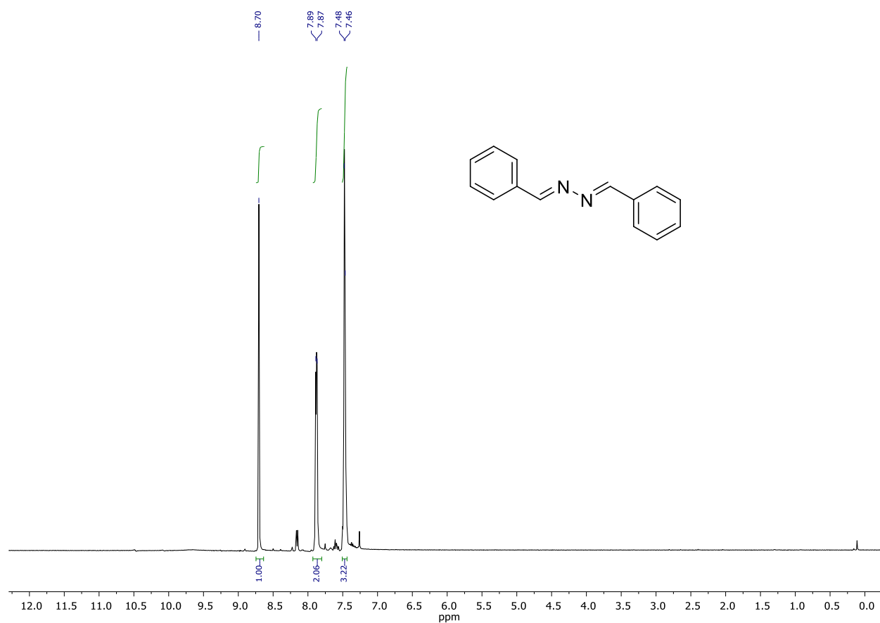
1 H NMR Spectrum of 1a (400.1 MHz, CDCl 3 )
