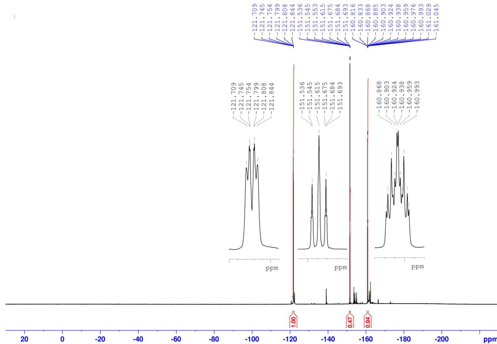
$^{13}\text{C}\{^1\text{H}\}$  NMR (75.4 MHz, C<sub>6</sub>D<sub>6</sub>, 298 K) of Al(C<sub>6</sub>F<sub>5</sub>)<sub>3</sub>·Pyridine complex
