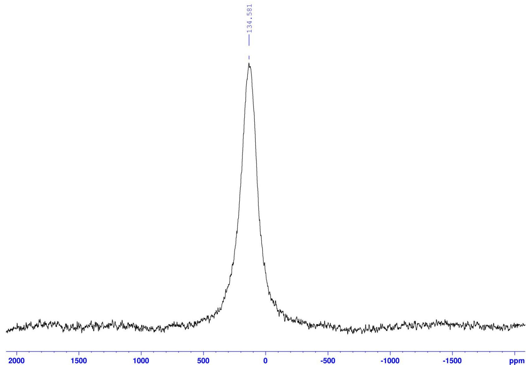
$^{27}\text{Al}$  NMR (78.2 MHz, C<sub>6</sub>D<sub>6</sub>, 298 K) of Al(C<sub>6</sub>F<sub>5</sub>)<sub>3</sub>·0.5toluene — Line shape analysis
