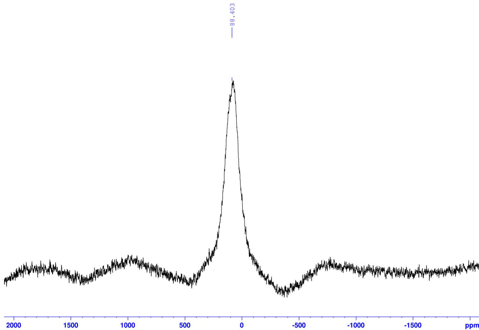
$^{27}\text{Al}$  NMR (78.2 MHz,  $\text{C}_6\text{D}_6$ , 298 K) of  $\text{Al}(\text{C}_6\text{F}_5)_3 \cdot \text{MeCN}$  complex — Line shape analysis
