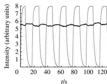
**Figure 2** Alteration of laser radiation due to switching off the magnetic field on the line of OH radical 2512 GHz. Dashed line shows the dependence of the magnetic field on time.
