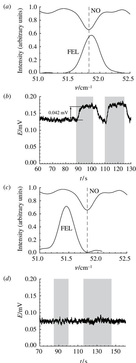
**Figure 1** Observation of Faraday effect in rotational spectrum of NO. (a), (c) FEL radiation spectra. Vertical line marks the position of NO absorption line  ${}^2\Pi_{3/2}$  ( $15.5 \rightarrow 2^1\Pi_{3/2}$  (16.5)). (b), (d) Alteration of radiation due to turning on the magnetic field of 8 kGs (gray areas).
